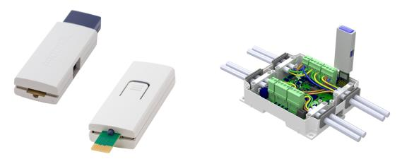
MyTool Connect is a Bluetooth dongle for connecting Produal MyTool® to a Produal device that doesn't have built-in Bluetooth connection. The dongle can also be used to power up the device for commissioning.
