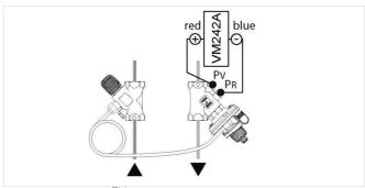
Requires SafeCon<sup>TM</sup> pressure test valves on both ports of Kombi-Auto
