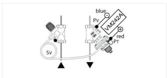
Requires SafeCon $^{TM}$  pressure test valve on lower connection of Kombi-Auto valve housing
