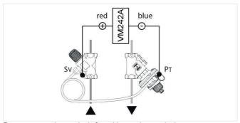
Requires a valve with defined kvs value with the pressure test ports in the supply, the pressure test ports must be designed across the valve seat for flow measurement e.g. Kombi-S with SafeCon pressure test connections.
