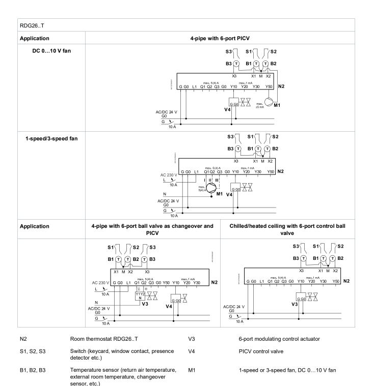
**Note**: In application "4-pipe with 6-port ball valve as changeover and PICV", Y50 can be connected with a DC 0...10 V fan.
