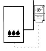
Low Limit For Frost Protection of Exposed Pipework
