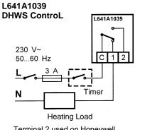
Terminal 2 used on Honeywell Y-Plan systems
