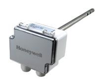
The HAVDT series is intended for use in commercial environments. It is designed with a duct mount probe and adjustable collar suitable for round or rectangular ducts. The transmitter provides separate readings for air velocity and temperature. It comes with three measurement ranges in a single device (0–2 m/s, 0–10 m/s, 0–20 m/s).
