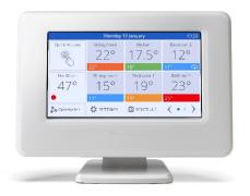
The evohome Central Controller is a multi-zone controller providing independent time and temperature control for radiator or underfloor heating systems as well as stored domestic hot water.
