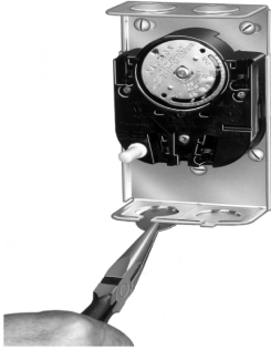
Fig. 5. Removing slotted knockouts.
