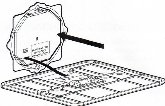
**EN** Push power module into wallbox with mains wiring to the rear.
