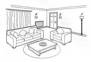
Position wall box at aheight of min. 1.2 m.
