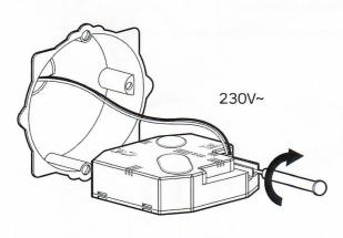
Insert wires into power module, observing correct polarity.
