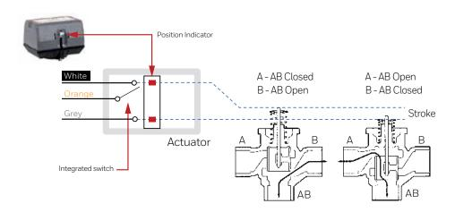
Please note when spring fully extends the valve stem A port is closed on both 2-way and 3-way valves. When actuator pushes in the valve stem against the spring load making it to retract fully, B port is closed on all valve variants.
