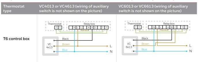
Honeywell Home wireless thermostats chronotherms are supplied with relay box having SPDT relay, the same type of relay box is used in Evohome zone system
